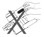
Do not place the appliance as above when removing or installing the HEPA filter, to prevent dust from entering the motor.
