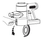
Press the release button on the side of the dustbin to empty the contents.
