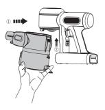
When re-attaching the dustbin, hold on an angle and slot the top of the dustbin into the hook on the main body. Push upwards until the hook is fixed into the slot on the dustbin and then it clicks back into place.
