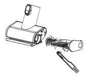
Remove the debris wrapped around the roller with the Tineco Hair Cleaning Tool.
